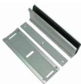
U-185 U Bracket Glass Door for KML-6, KML-10 (x2) & KML-2H - Suits 10-12mm thick glass 185L x 62W x 33D(mm)
