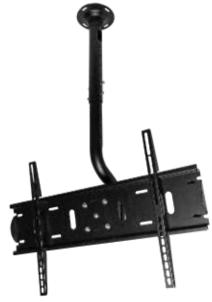
A heavy duty ceiling mount bracket suitable for mounting flat screens up to 75kg. The swivel mount allows 15° of vertical tilt adjustment and 130° of horizontal adjustment. The design enables adjustment to suit screens up to 800x500 VESA mount size. Mounting height from ceiling can be varied 100mm steps up to a max of 1.2m from ceiling (to
