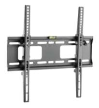
Offering tilting functionality (-8°) for screens installed at raised heights. Low profile design, just 40mm from surface. Includes spirit level for easy installation. Dual pull safety lock ensures TV cannot come off the backing plate without both locks being simultaneously released. Note: Due to the ultra low profile of these brackets, it is best used in combination with a recessed power point (such as P 8058).
