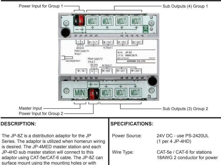
surface mount using CA1-5e/CA1-6 cable. The JP-82 can surface mount using the mounting holes or with the W-DIN11 mounting rail. One or two PS-2420UL power supplies are used, depending on how many sub master stations are connected.
