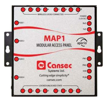
To simplify installation, support and maintenance, the MAP1 contains twenty seven status LEDs which show, for example, AH30 hubs connected, locks connected, lock/unlocked state of each lock, power and several others.
