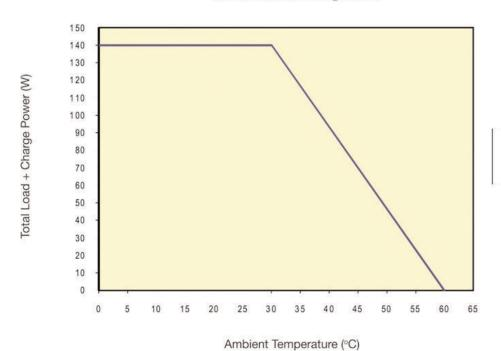
PB256-1210CML/2405CML Attached to 300x300x2mm Al-Plate
