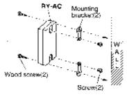
For wall mounting, attach unit to wall with supplied mounting hardware.
