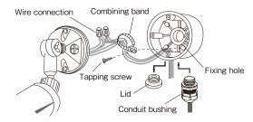
(4) Fix the mounting base tightly to the mounting box by the 2 screws.
