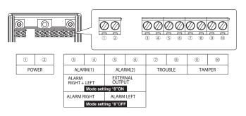
POWER: 9 to 28V DC (non-polarity) Current consumption 30mA Max. ALARM OUTPUT (1) : 30V (AC/DC) 0.2A Max. (Resistive load), N.O./N.C. selectable ALARM OUTPUT (2) : 30V (AC/DC) 0.2A Max. (Resistive load), N.O./N.C. selectable
