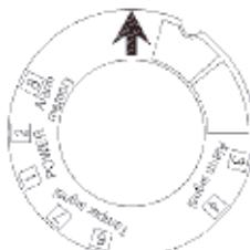
①---② Power (non-polarity) N.C. contact : 25mA or less
