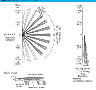
Detection distance is set by adjusting the angle of downward zone Adjustable range 10' (3m) to 40' (12m). [9 ranges]
